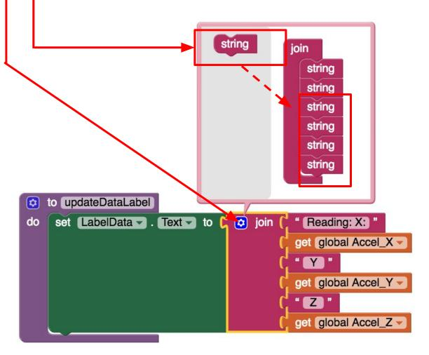
Finally, we need to call the procedure when this data is received.
